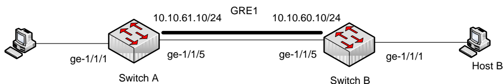
Figure 4-2. GRE tunnel configuration
