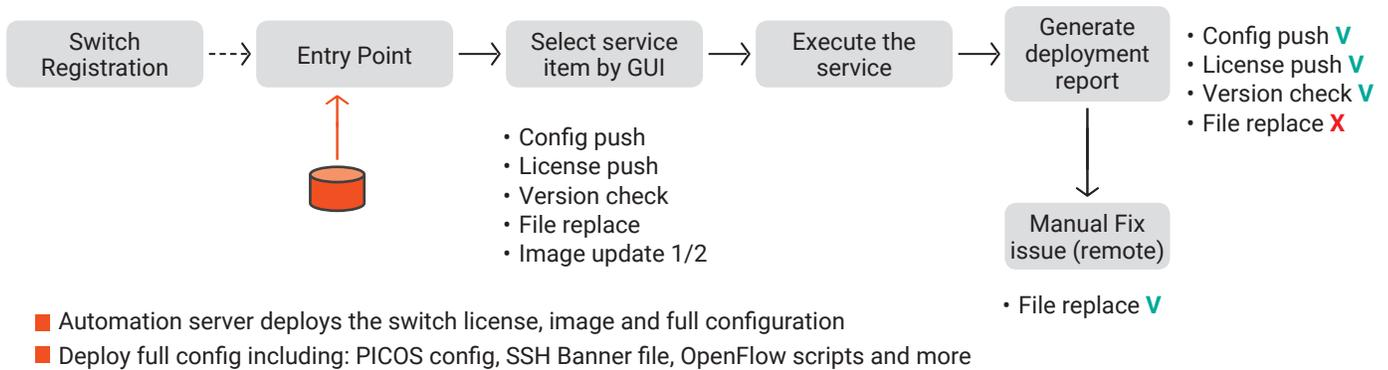
The automation process described above in Figure 6 can be applied simultaneously to dozens of switches being deployed across the same or different sites in the customer network. In practice, this supports a deployment rate of several hundred switches per week. (Actual scalability depends on the CPU and RAM in the VMs being used.) The automation server is designed for high availability with full active-active redundancy across two instances of the server and database.
